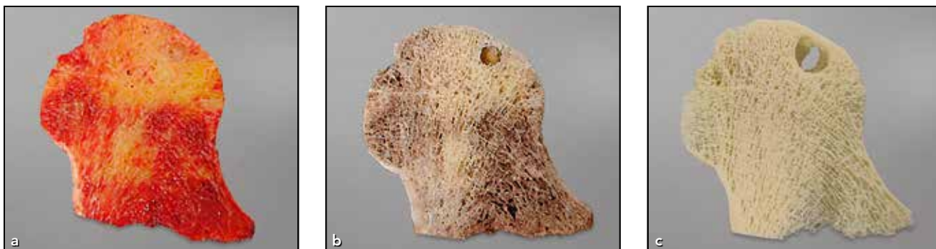
Fig 1 Supercritical CO 2 procedure showing the trabecular bone tissue (a) before, (b) during, and (c) after cleaning, with the initial architecture and volume retained at the end of the process.
